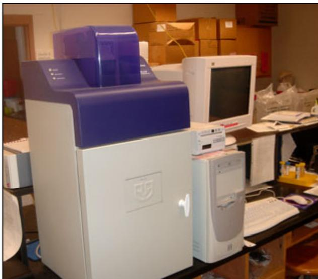
Figure 1 – AutoChemi Imaging System
