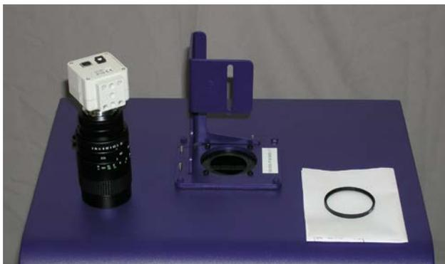
1. Align the holes of the gasket and base. Attach the base and gasket to the darkroom using the screws provided. Position the bracket on the mounting base aligning the holes on the base. Using the four thumb screws provided, secure the bracket to the base.
