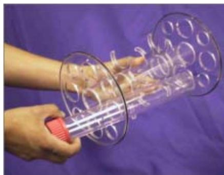
**WARNING:** Do not insert a bottle into the center tube. To do so would block air flow and may result in a safety hazard and or malfunction.
