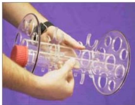
4. Open the HybriCycler's door by pressing down on the rear portion of spring-loaded door latch. Slide the bottle carousel into the hybridization chamber ensuring that the front disk is inserted into the groove of the carousel guide. Close the door by squeezing the door against the hybridization chamber until the spring-loaded door latch secures.
