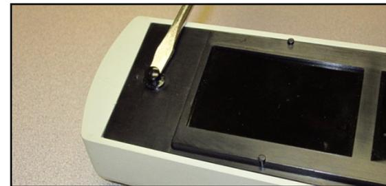
To replace the filter frame, slide the large part of the frame into the lower end of the lamp housing. Press the frame into position and snap the nylon button inward to the locking position.
