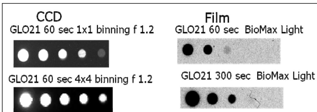
**Figure 4.** CCD and film exposure by a calibrated light source, GLO21, to compare sensitivity. A five-step GTLS calibrated light source (GLO21) was used to compare sensitivity between the BioSpectrum 500 system and typical chemiluminescence optimized film. The GTLS standard covers a 600 fold range from most intense (left) to least intense. The film cannot record the weak signals from the standard, while the CCD can quantitate all five intensities in 60 seconds or less.
