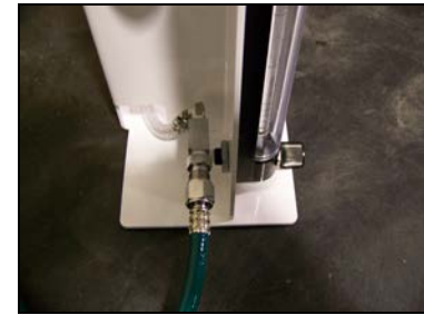
Figure 2: Attach Oxygen Source to Vaporizer Stand Input
