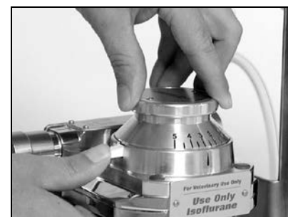
Figure 10: Adjusting the Vaporizer Dial
