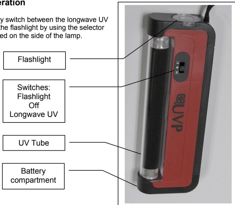
Insert 4 AA batteries (UM-3) not included with the lamp. To insert batteries, slide the battery cover out and flip upwards. Position the batteries as shown on the inside of the battery compartment. Slide back the battery cover.
