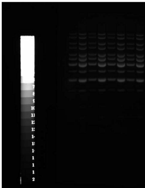
**Figure 9.** Captured image showing sample ethidium bromide stained DNA gel and calibration step tablet at 0.5 second exposure.
