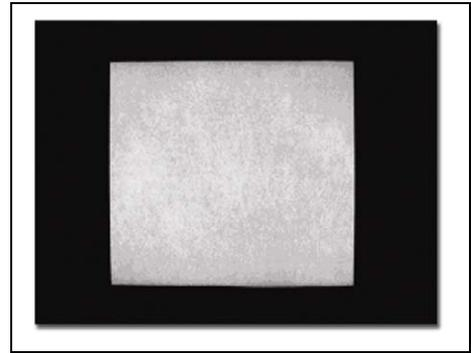
**Figure 2.** FirstLight UV Illuminator shows <5% CV
