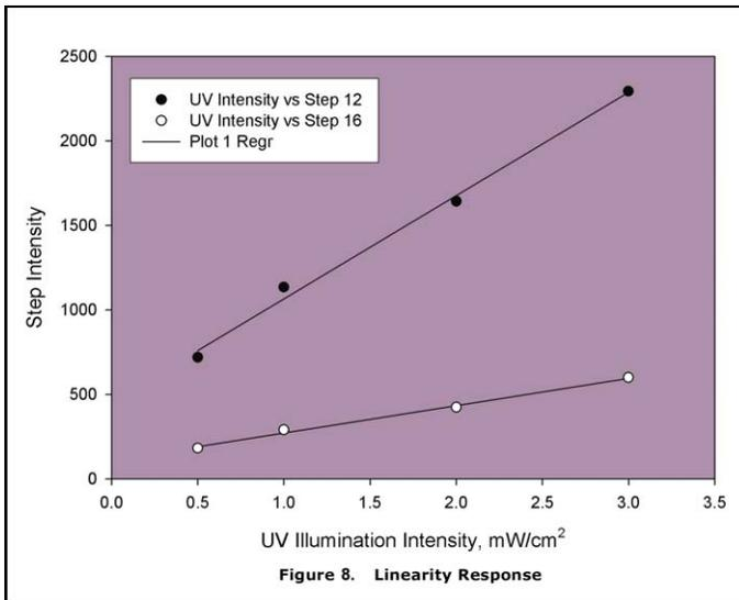
**Figure 8.** The step tablet responds linearly to increases in UV intensity. The response of steps 12 and 18 to increased UV intensity using a variable intensity FirstLight Illuminator are shown. UV Intensity at 302 nm was measured using a UVP NIST traceable UV calibration meter (**UVX-31**).
