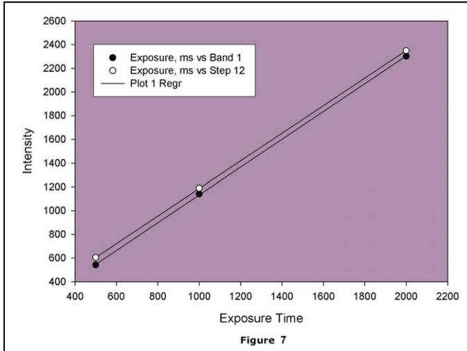
**Figure 7.** The step tablet responds linearly to increases in UV exposure. Exposure time and intensity comparison of DNA Band 1 (lane 2) from the gel and Step 12 from the Fluorescent Calibration Step Tablet in figures 9 and 10 above. Note the increased exposure leads to simultaneously a brighter image of the DNA fragment and Step 12 of the calibration tablet. Step 12 is also good substitute for a typically stained fragment of DNA.
