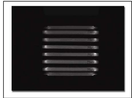
**Figure 3.** M-26X Transilluminator is very uneven and shows 81.8% CV Full Area, 84% CV Inner Area
