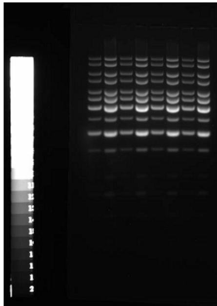
**Figure 10.** Captured image of the same sample DNA gel and calibration step tablet from figure 9 above except with a longer 2-second exposure. Note both the DNA bands and the step tablet increased by the same percentage (figure 7).
