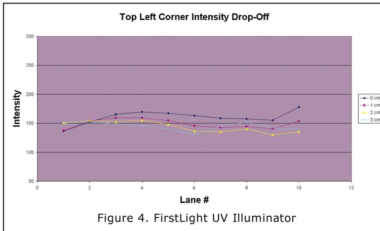
**Figure 4 and 5.** Intensity Profile of electrophoretically separated Protein Standards: Comparison of FirstLight Illuminator and 8-Watt Transilluminator. Equal amounts of protein were loaded per lane, stained with SYPRO Ruby, and the individual protein fluorescence intensity was quantitated. Note the severe loss of signal toward the edge of the typical nonuniform UV light table (Figure 5) compared to the uniform FirstLight illuminator (Figure 4).
