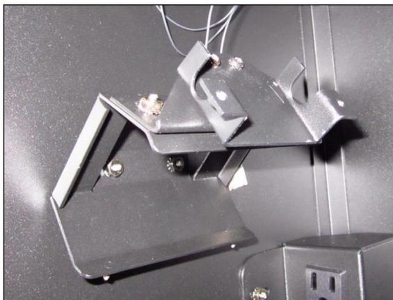
2. Thread the knurled (non-smooth side) of the fiber optic cable from the inside of the darkroom through the hole created by removing the stopper until the large bulb separating the smooth and rough side of the fiber optic cable can no longer be pushed through the opening.
