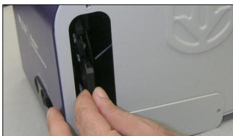
3. To access the other filter positions, manually rotate the filter wheel with the eLITE powered off.
