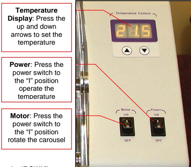
**Temperature Display:** Press the up and down arrows to set the temperature
