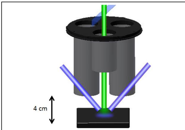
**Figure 4.** Working distance from stage to optics (4 cm) in the iBox Explorer<sup>2</sup> Imaging Microscope. Typical working distances (imaging stage to objective) for most microscopes average 0.1 to 4 mm, limiting both the field of view for imaging as well as the size of the sample that can be placed on the stage.
