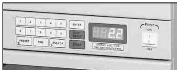
Crosslinker Control Panel
